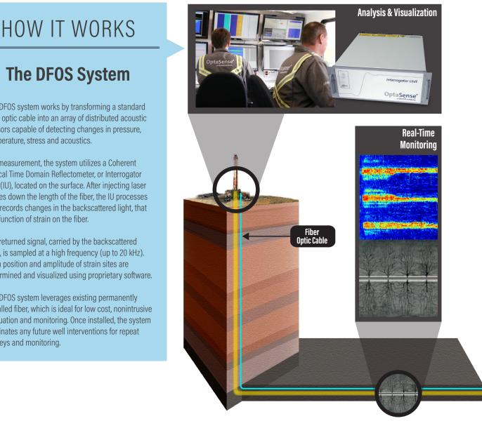
The DFOS system works by transforming a standard fiber optic cable into an array of distributed acoustic sensors capable of detecting changes in pressure, temperature, stress and acoustics.
